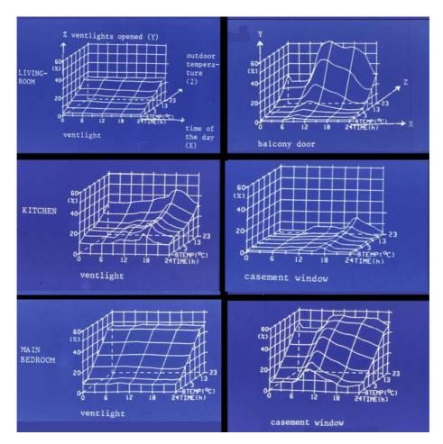
**Figure 1** The use of ventilation provision (total % opened windows or vent lights in 80 apartments in a ten storey high flat-building) (Y axis) as a function of outdoor temperature (Z) and the time of the day (X). Shown are the use of the ventlight and the balcony door in the living room (row on top), the use of the provisions (vent light and casement window) in the kitchen (second row) and in the main bedroom.
